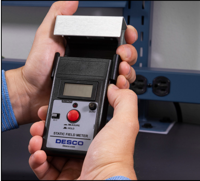
Figure 8. Sliding the Conductive Plate onto the Digital Static Field Meter
