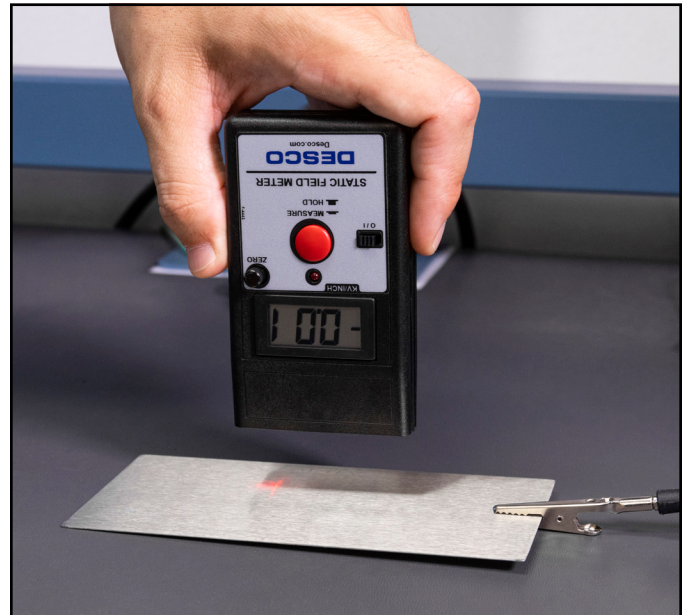
Figure 6. Pointing the Digital Static Field Meter to a grounded surface
