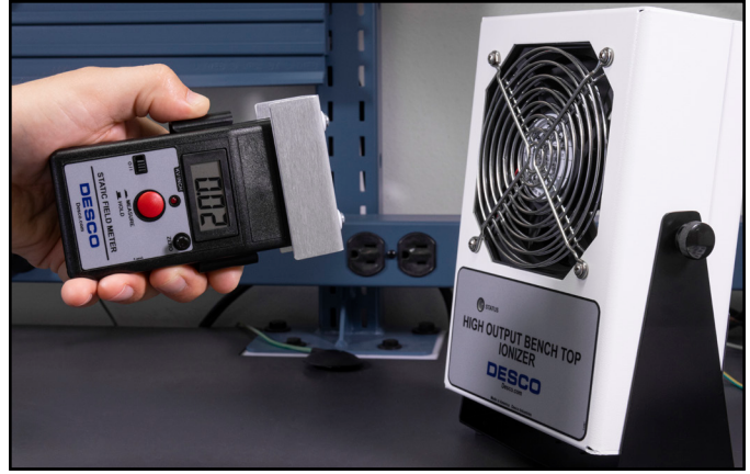
Figure 9. Using the Digital Static Field Meter with Conductive Plate to measure the offset voltage of a benchtop ionizer
