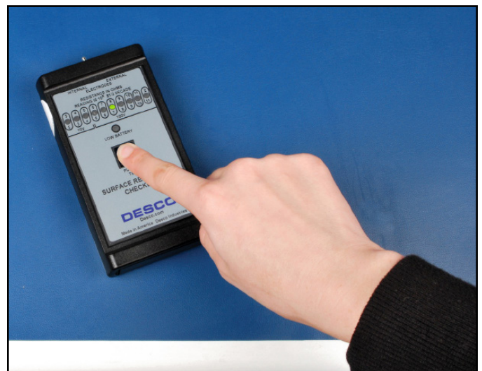
Figure 3. Using the parallel electrodes to measure surface resistance
